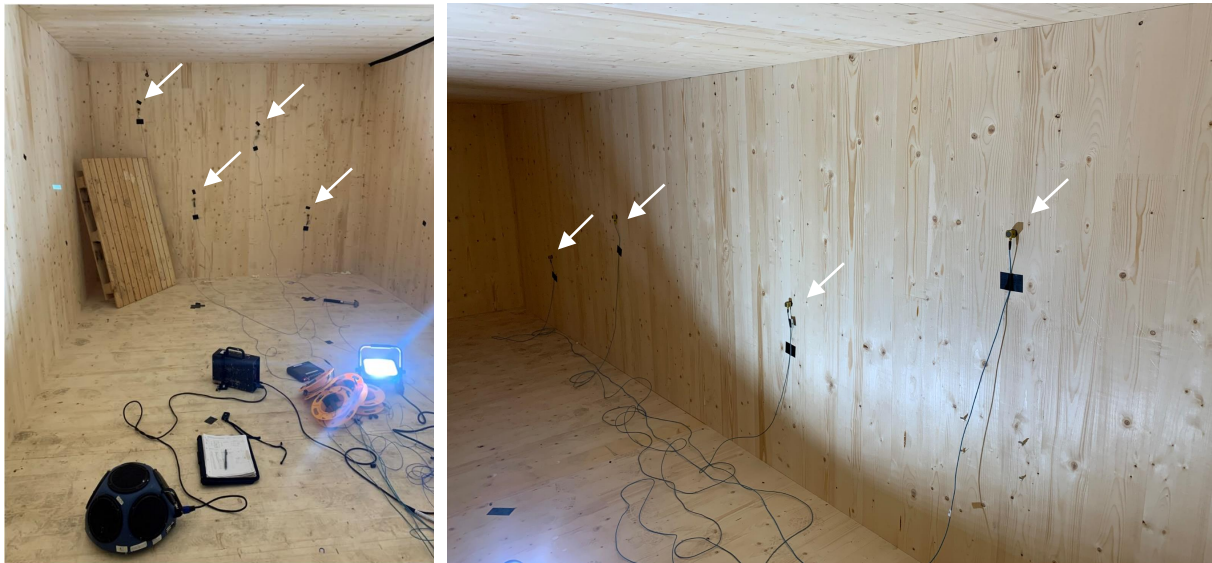
Figure 3 – Photo of sensor setup inside of the test rooms. Sensor positions indicated with white arrows.
