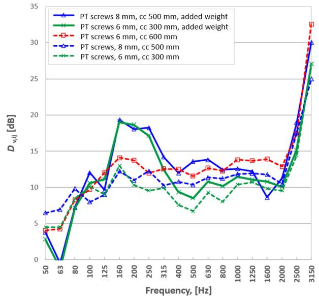
**Figure 7.** Measurement results of horizontal attenuation with screw fasteners of various type and spacing. Solid and dashed lines show results with and without added mass, respectively.
