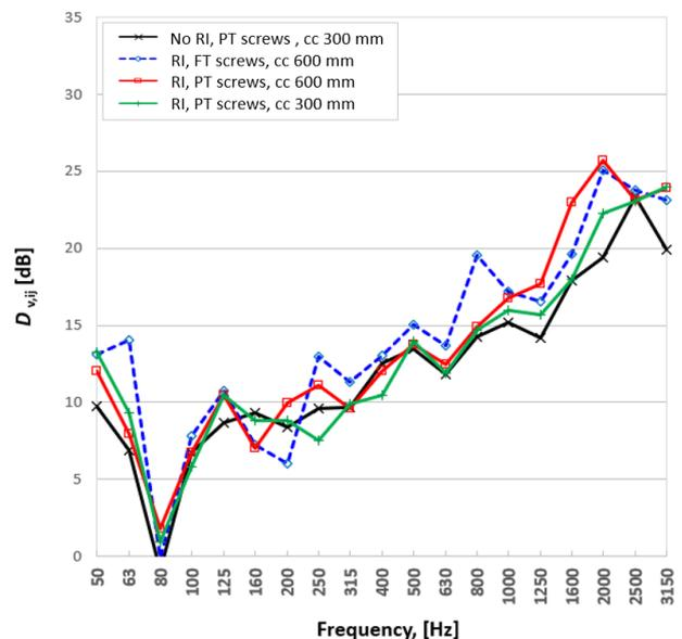
**Figure 8.** Measurement results of vertical attenuation with screw fasteners of various types and spacing, where solid and dashed lines indicates partially (PT) and fully (FT) threaded screws, respectively.
