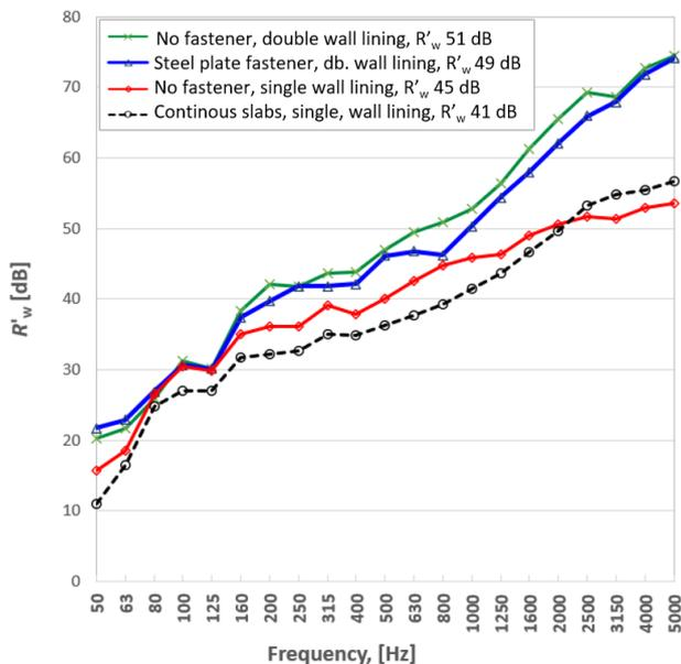
**Figure 9.** Airborne sound insulation between the horizontally adjacent rooms. Solid lines show results with walls and roof cut, as indicated in Figure 10. The green and blue line is measured with wall lining also in the receiver room.
