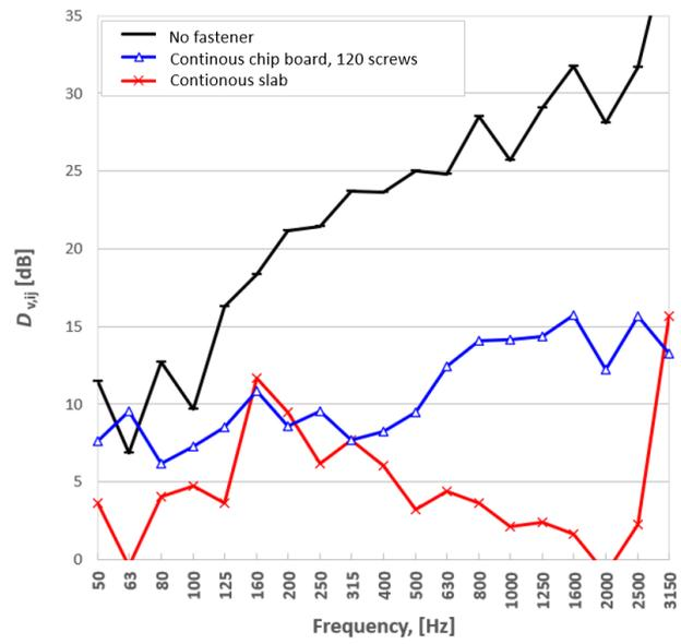
**Figure 5.** Measurements of vibration level difference between roof slabs in horizontally adjacent rooms. The red line shows results with continuous CLT wall and slab elements, black line with a full wall and roof slab cut, and blue line with a chip board across the roof split as seen in Figure 4b).
