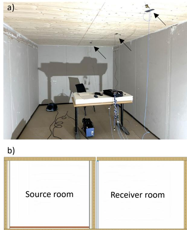
**Figure 3.** a) Photo of sensor setup inside of the test rooms (only 3 of the 4 sensors visible in the photo). Sensor positions indicated with arrows. b) Schematic of the test set-up, also indicating the cut in the roof slab and the additional columns.
